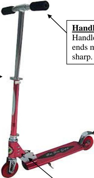
**Handlebars.** Must not be loose. Handlebars should have grips and the ends must be covered as they can be sharp.
